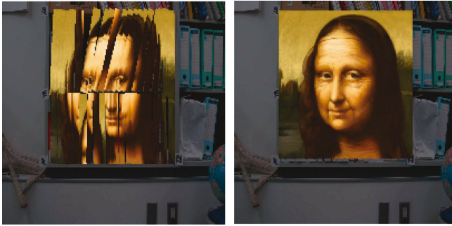
Fig. 6. Two example outputs of the Mona Lisa Bookshelf. The image on the left shows that some books are tilted and in the wrong order. Some books are also missing. The image on the right side indicates that none of books have been picked up for a long time.
