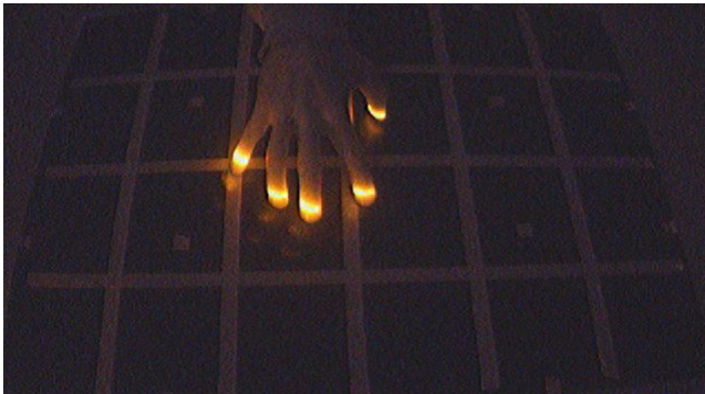
Fig. 5. Image seen by the camera. Visible light is filtered out using a 800nm pass filter.
