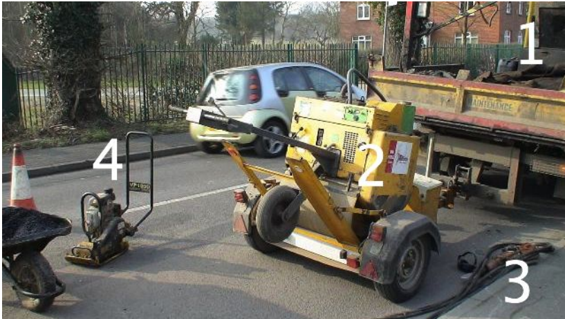
Fig. 1. Key Equipment Used for Road Patching: 1 – Van, 2 – Petrol Powered Drum Roller/Air Compressor (Stored on Trailer), 3 – Air-powered Pavement Breaker, 4 – Petrol Powered ‘Wacker’ Plate Compactor
