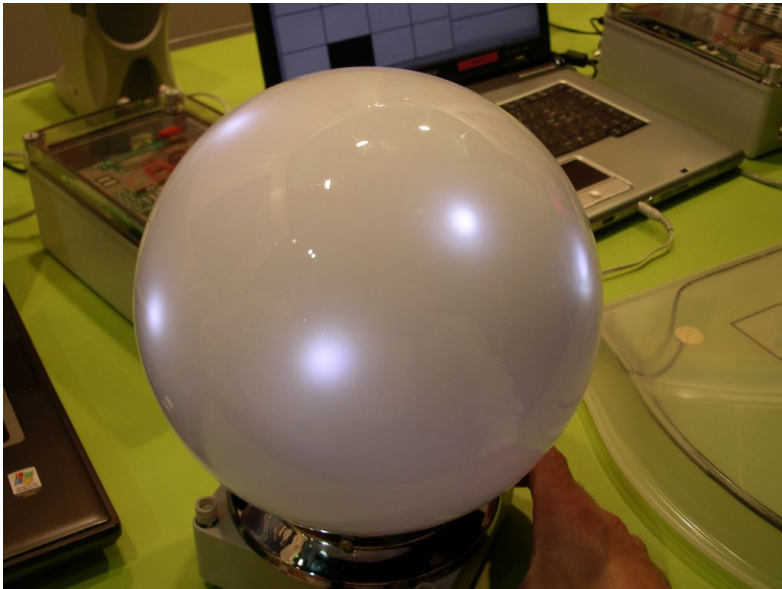
Fig. 6. The light globe with LED's placed under the surface and indicating the position of sensitive spots
